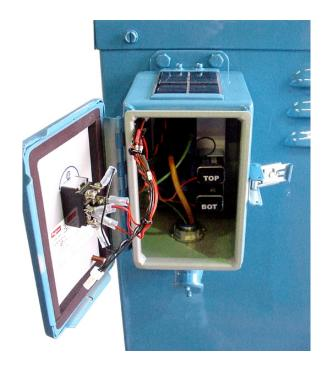
Unit operated by two 9V batteries and Solar Panel.
